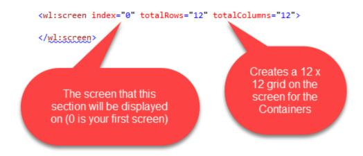
We have not defined the size of the columns or rows, instead Myriad will take the screen resolution and divide it into the amount of rows and columns required. This means that the layout will work on standard and wide screen monitors and on monitors with different resolutions, however, you may wish to create different Dynamic Layouts for use on PC's with widely different screen types or configurations (for example screen in portrait mode).
