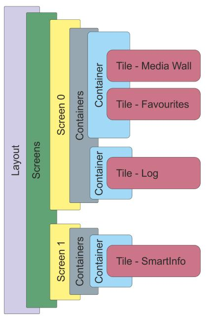
**Layout Node** – This is the overall Dynamic Layout and should be the first and last tags in your Dynamic Layout File.
